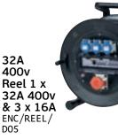
Inlet: 32A 400v Length: 25m 6mm 5 core Outlets: 1 x 32A 400v, 3 x 16A 230v Protection: 3 x 16A SP MCB, 1 X 40A 30mA RCBO
