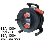
Inlet: 32A 400v Length: 25m 6mm 5 core Outlets: 2 x 16A 400v Protection: 2 x 16A 4 Pole MCB, 1 x RCD 40A 30mA
