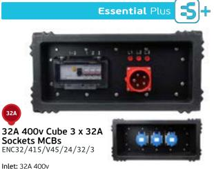
Outlets: 3 x 32A 400V Protection: 1 x 40A /30mA 4P RCD, Type A 3 x 32A 1P MCB, C Curve Enclosure: V45/24, IP44
