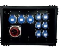
Inlet: 63A 400v Outlets: 3 x 32A 230v & 6 x 16A 230v Protection: 6 x 16A /30mA RCBO Type A 3 x 32A/30mA RCBO Type A Enclosure: Titan Cube V45/36, IP44
