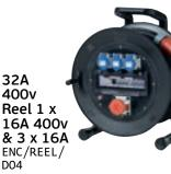
Inlet: 32A 400v Length: 25m 6mm 5 core Outlets: 1 x 16A 400v, 3 x 16A 230v Protection: 3 x 16A SP MCB, 1 x 16A 4P MCB. 1 X 40A 30mA RCBO
