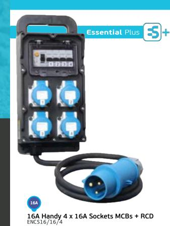
Inlet: 16A 230v with 2m Cable Outlets: 4 x 16A Protection: 1 x RCD 40A /30mA, 2P Type A 4 x 16A MCBs 1 Pole C Curve Enclosure: S06 Handy Board, IP44
