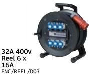
Inlet: 32A 400v Length: 25m 6mm 5 core Outlets: 6 x 16A 230v Protection: 6 x 16A SP MCB, 1 x RCD 40A 30mA
